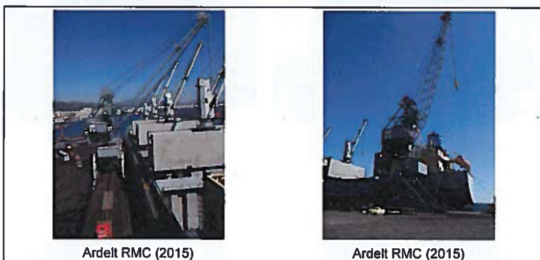
Figure 7: Rail Mounted Harbour Crane Ardelt
