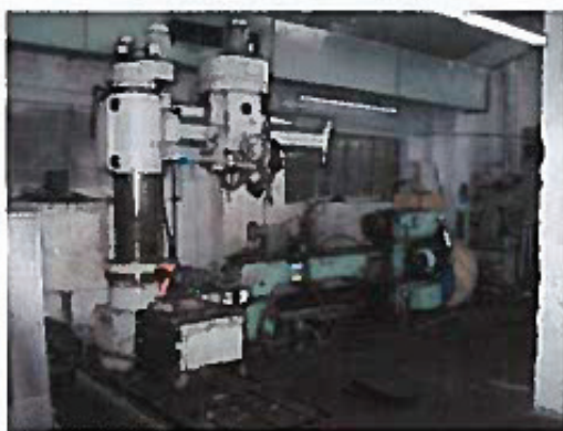
Workshop Bulk and General Cargo – Lathe and radial drilling machine used in workshop
